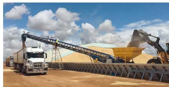
Outloading via BunkerStacker3000 fitted with surge hopper
