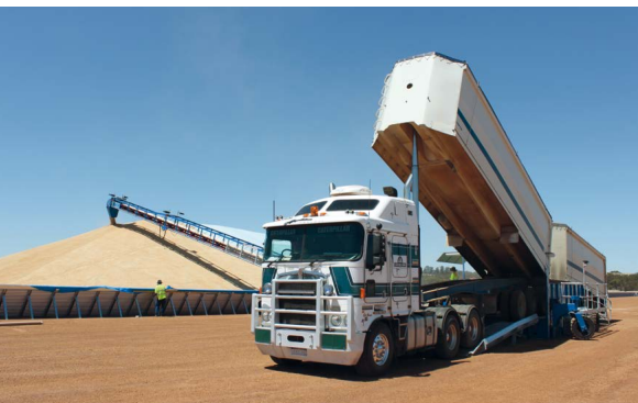
Drive Over Hopper in operation – B-double trailer
