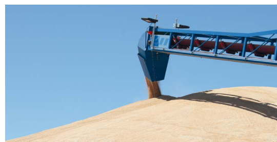
Stacker filling bunker
