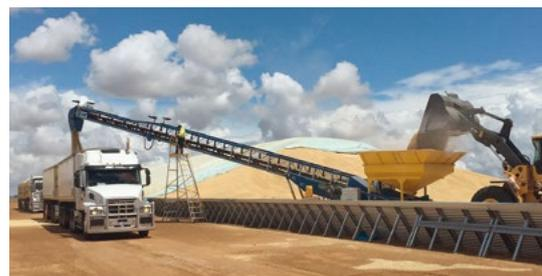
Outloading via BunkerStacker3000 fitted with surge hopper
