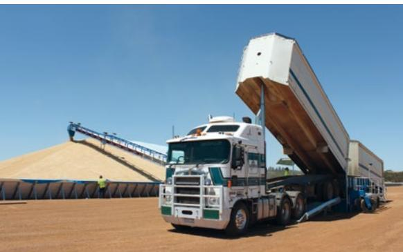
Drive Over Hopper in operation – B-double trailer
